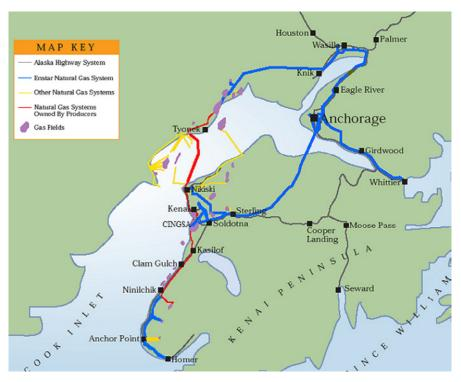
Buried in rights-of-way, these transmission pipelines range from 2" to 20" in diameter and are made of high strength steel. They operate at pressures from 270 to over 1,000 pounds per square inch (PSI).
